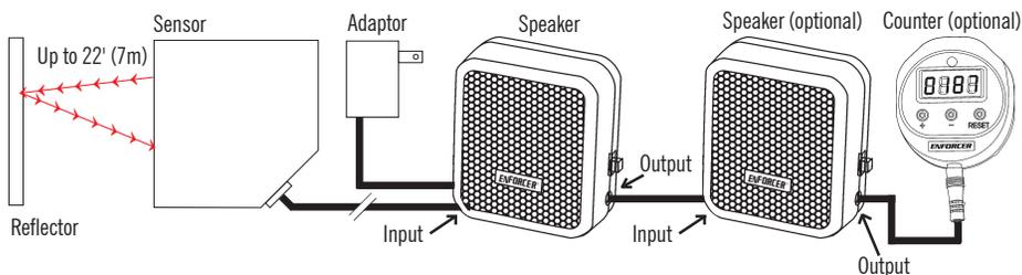
**NOTE:** a) When adding a 2nd speaker. If the application distance between speakers exceed 33 ft. (10m), then a power adaptor is required for the 2nd speaker.
