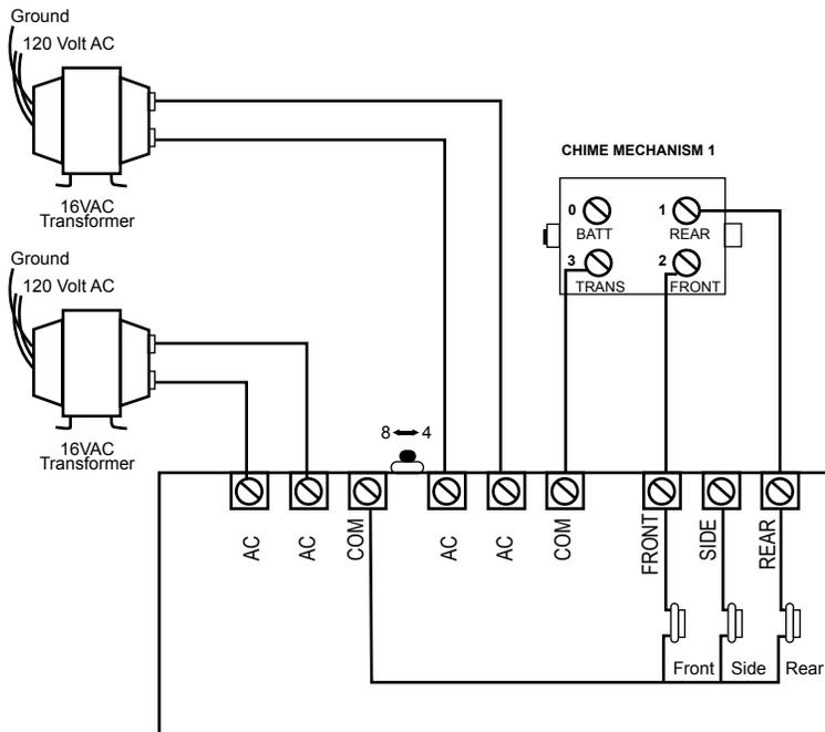
7. Turn on power at breaker box. Make sure pushbuttons operate chime properly. (Adjust switch on circuit board for 4 or 8 chime tones at front door. Side and rear doors will have 1 chime tone each.)
