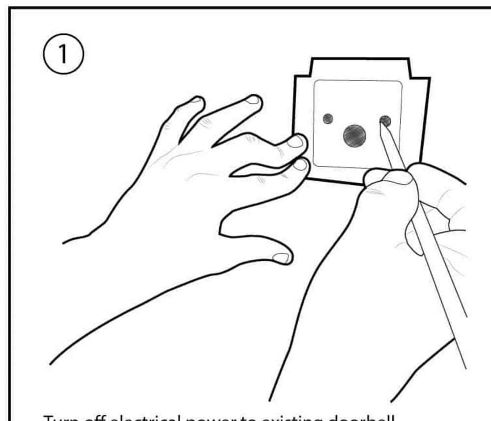
Turn off electrical power to existing doorbell. Remove old doorbell button. Use template provided to mark hole positions.
