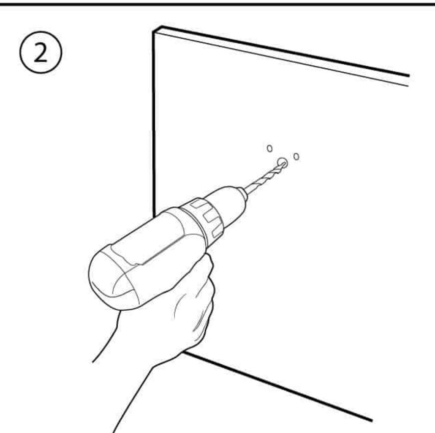
Drill holes using the appropriate drill bit for your surface material
