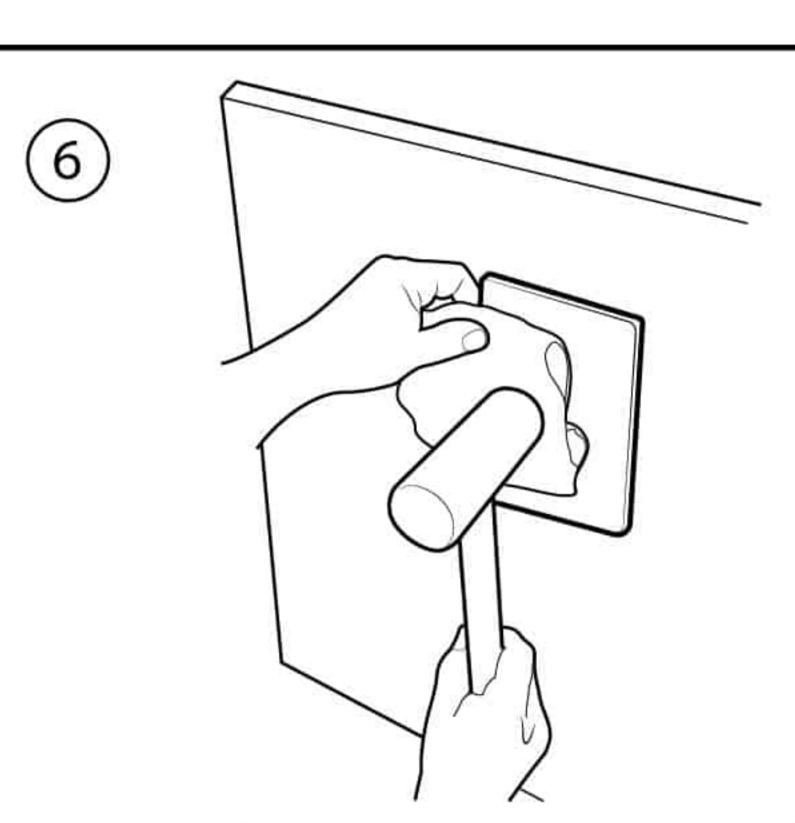
Using a soft cloth to protect the surface of the doorbell, GENTLY tap the posts into the plastic anchors, alternating sides, using a plastic or rubber mallet until doorbell is flat against the mounting surface. DO NOT HIT THE CENTER PUSHBUTTON WITH THE MALLET.
