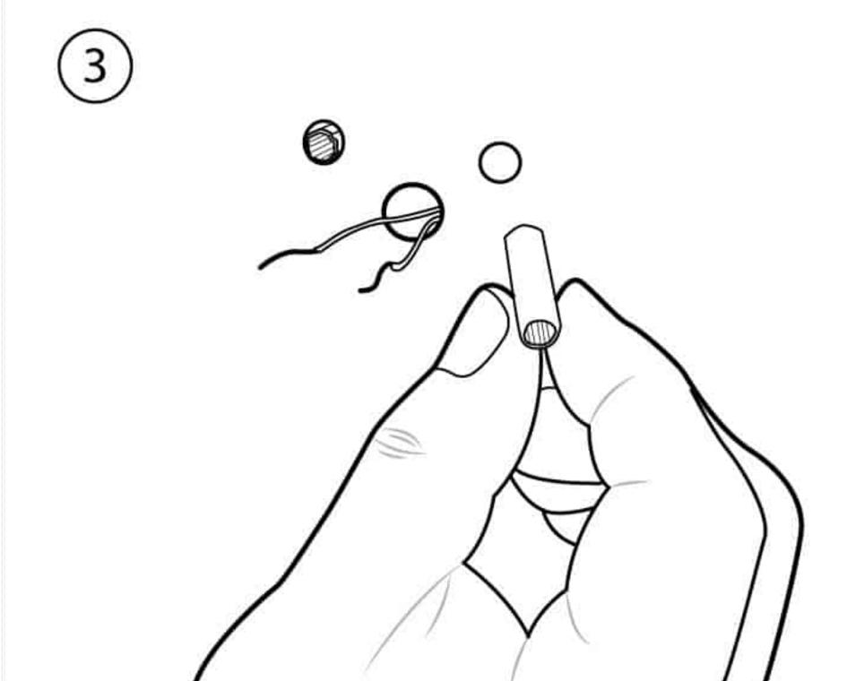
Insert plastic anchors into small holes
