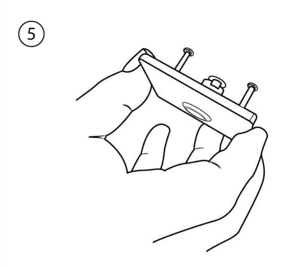
Push posts on back of doorbell into the plastic anchors
