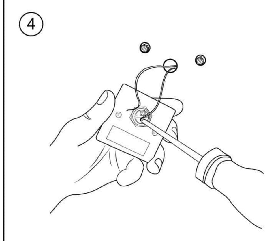
Attach wires to the 2 screw terminals on pushbutton
