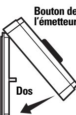
1. Place Chime Button where desired and mark screw locations.
