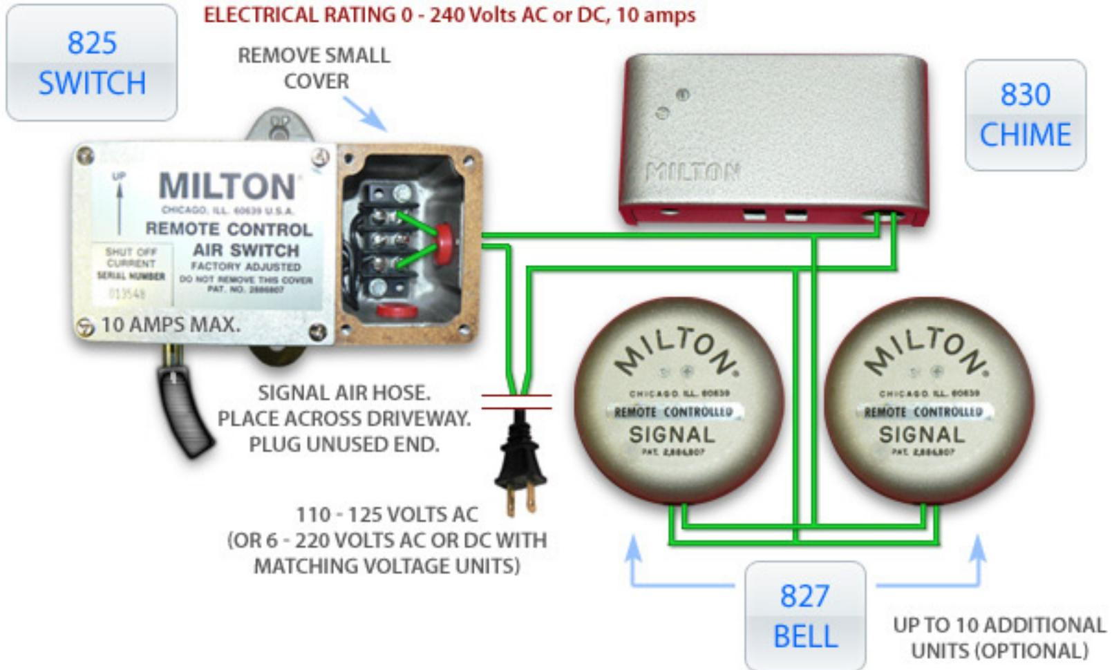
This is a pictorial wiring diagram to suggest various hook-up options and to show a typical circuit path. Any installation must be properly terminated and insulated and must conform to all applicable codes. Consult a qualified electrician. NOTE: The center terminal on the terminal strip can be used as a convenient tie point if desired.
