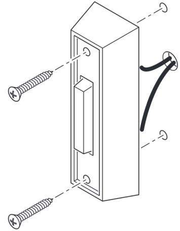
Use a screwdriver to remove wires mounted to existing push button.
