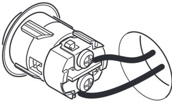
Connect wires from wall to push button screw terminals. *Note:* It does not matter which wire is connected to which screw.
