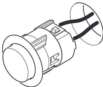
Attach push button to wall with screws provided (if applicable).
